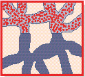
b) Plugging a plane in the capillary system → water movement stopped.
