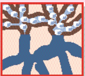
e) Hydrophobicity with narrowing of capillaries → water movement dramatically reduced.
