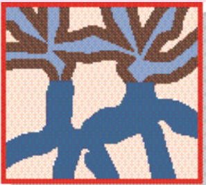
c) Narrowing of capillaries → water movement reduced.
